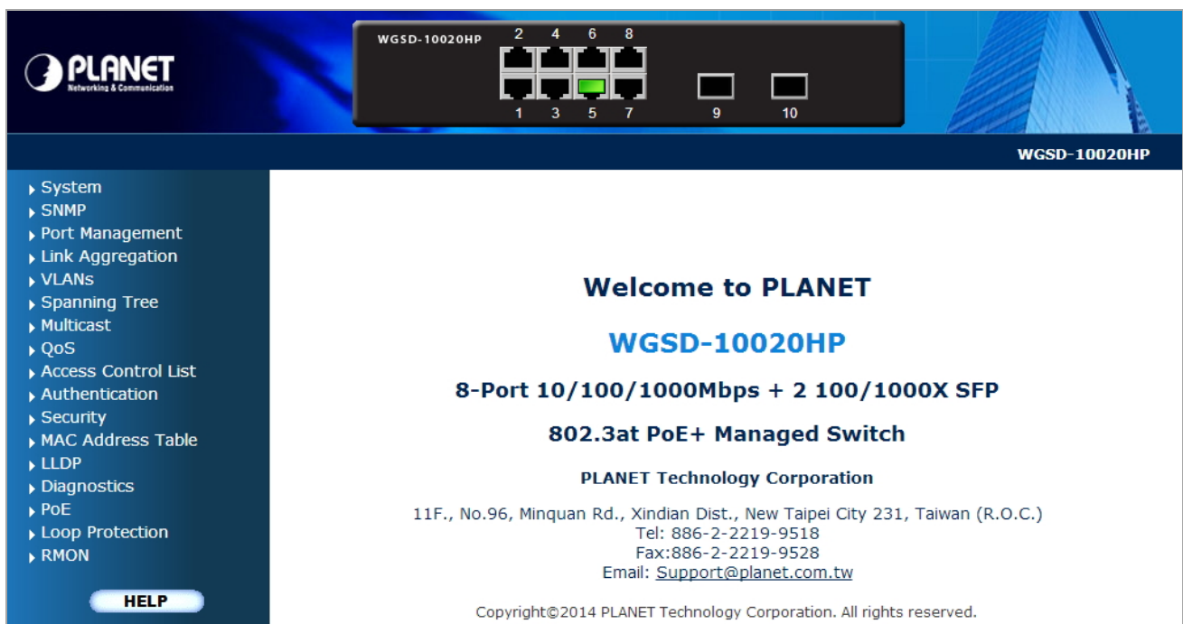
Figure 3-1-4: Web Main Screen of Managed Switch
